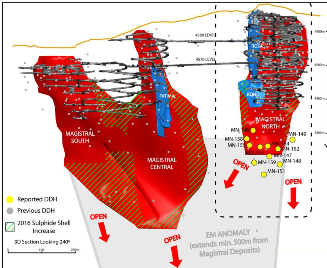
**Figure 1:** Cross section looking west showing Magistral Deposits with drill hole intercepts
