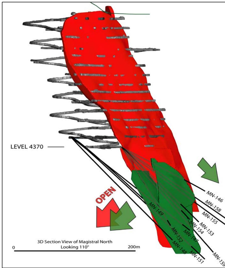
**Figure 2:** 3D view, looking southeast, and cross section illustrating geometry of the Oyon mineralization and location of recent drillhole intercepts in the Magistral North Deposit at the Santander Zinc Mine.
